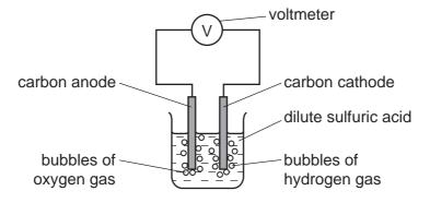
A reading on the voltmeter shows that electrical energy is being produced. Suggest an explanation for how this energy is produced.
